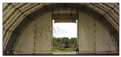
*Figure 10: Wide-span large capacity fabric shelter.* Images courtesy Weatherhaven.
